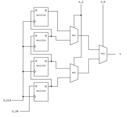
Note that  $S_{in}$  is a one bit signal and  $S_{clk}$  is only used for configuration.
