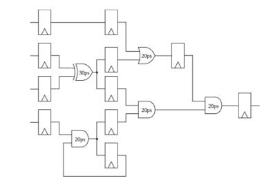
*Note*: The following diagram is wrong because it merges two FFs at the fanout of XOR gate even though we are not given initial values of FFs.
