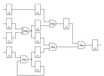
*Note*: The following diagram is wrong because it merges two FFs at the fanout of XOR gate even though we are not given initial values of FFs.
