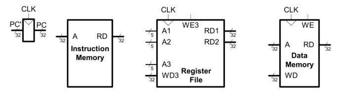
Note: for now, and for these state elements, clock is used for write but not for read (asynchronous read, synchronous write).
