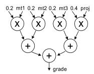
This time-multiplexing performs the action of each node one at a time.
