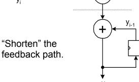
Pipelining is limited to 2 stages.
