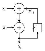
Can we "cut" the feedback and overlap iterations?
