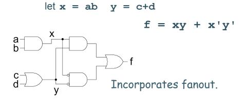
No convenient hand methods exist for multi-level logic simplification:
